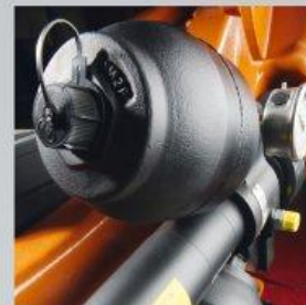
Extremely compact hydro-pneumatic counterbalancing system. 1
